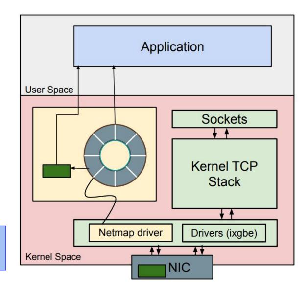
DPDK, netmap manage processing till L2 of network stack
